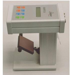
After a certain operating period, the parameters of the LED block can change (e.g. caused by temperature drift of the LED or intensity ageing). During the current operation this is compensated via the calibration on the hinged reference plate.
